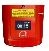
Intuitive and user-friendly display that shows battery level, curing time and if the fan is running. It also indicates if the temperature is too high and when service is required.
